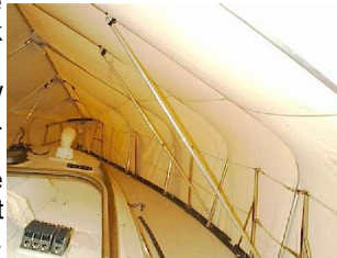
Shows ribs with braces
